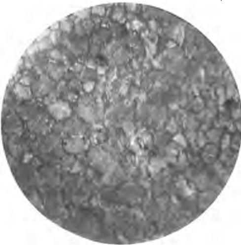
PHOTOMICROGRAPHS OF STEM OF TENSILE SPECIMEN C2-J', NO. 7636, CROSS SECTION. 16-INCH BY 18-INCH CARBON STEEL INGOT. MAGNIFICATION OF EACH 53 DIAMETERS. STEEL HEATED WHITE HOT AND QUENCHED IN BRINE.
